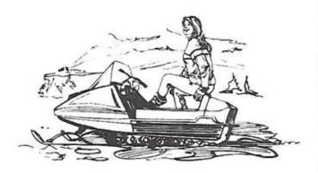
portant thing to remember before you contemplate such a trip is to know your machine. Learn to change a spark plug and drive belt. Carry the proper tools for your sled, as well as a flashlight, knife and some good, strong tape (duct tape works great for many things). Also make sure that you carry a tow rope.
